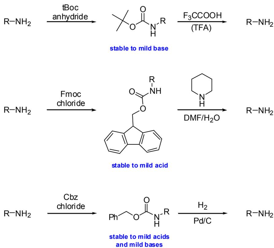
Take note of orthogonal protecting groups that are removed with different conditions so you can selectively deprotect one group at a time
